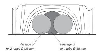
The images are only for examples. Recyclable material is allowed a size tolerance of  $\pm$  1,5%.
