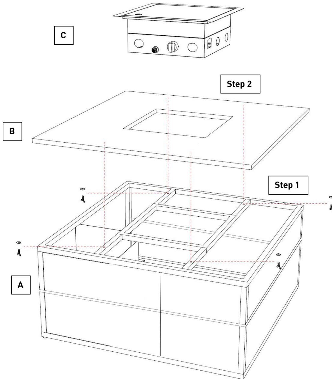
Package 1 / Pakket 1: Frame (A) and burner (C) / Frame (A) en brander (C)
