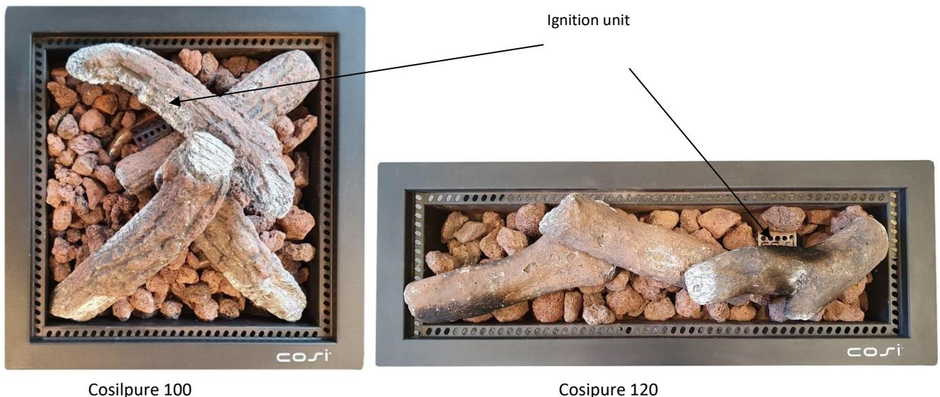
Keep the space around the ignition unit free of lava rocks. Make sure the fire ring and ignition unit are only minimally covered by the logs. If the logs block the fire ring, dangerous situations may occur. The blockade of the fire ring will affect the air flow of the ring and the flames will be different. This results in dangerous situations!
